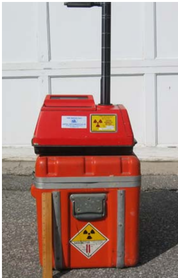
Figure 8: A portable nuclear gauge
